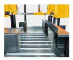
Dual Vise The machine equips a hydraulic full stroke dual vise clamping system.
