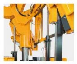
Cylinder with Auxiliary Square Post The design of cylinder with one auxiliary post allows for lifting the saw frame to achieve maximum stability, making the machine excellent for heavy duty cutting. (H-560HA)
