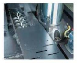
Automatic Chip Conveyor The device delivers chips to a tank located at the outside of the machine. This helps to maintain a clean interior for the machine. while saving time in manual chip removal.
