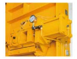
Hydraulic Blade Tension The saw blade tension is controlled by hydraulic power, allowing the saw blade to maintain a proper tension at all times.
