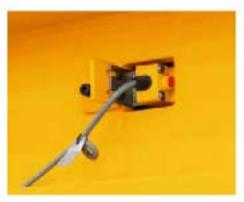
Blade Breakage Detector If any blade breakage occurs during cutting, the machine will automatically stop to ensure safety of aperator and machine.
