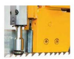
Out of Square Detector (Option) The out of square detecting value can be set. Once the detecting value exceeds the setting value, machine stops automatically.
